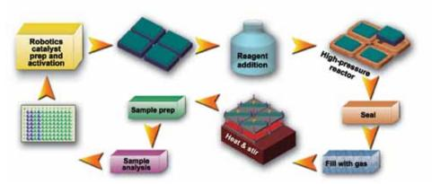
The Combinatorial Catalyst Laboratory (Combicat) is an integrated system for high-throughput catalyst experimentation at near-processing conditions, as can be seen in this schematic. This combination of high-throughput and processing conditions is unmatched at universities or other national laboratories.
