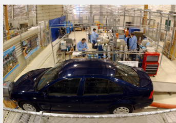
In the Exhaust Emissions Science Laboratory, we investigate methods for reducing engine emissions from more fuel-efficient future vehicles.
