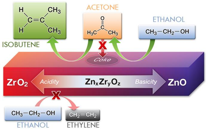
The right balance of zinc and zirconium oxides in this catalyst (purple block) converts ethanol to isobutene with low amounts of unwanted byproducts such as acetone and ethylene.
