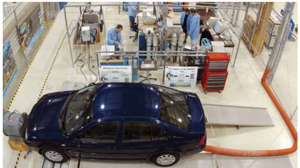
Researchers in PNNL's Engine Emissions Laboratory investigate catalysts, particulate traps, and other methods for reducing diesel engine emissions.
